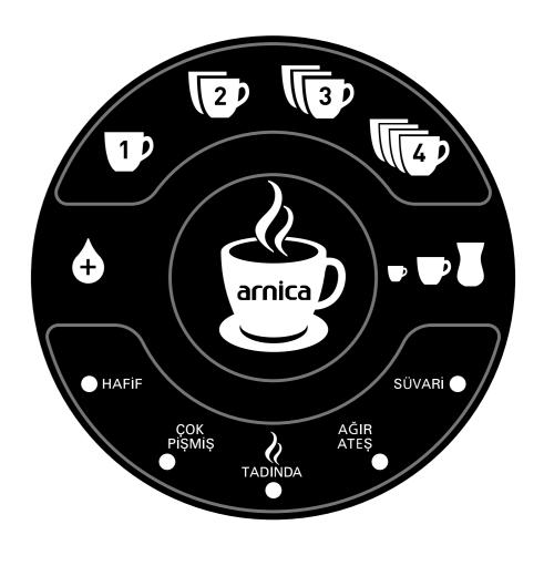
The user puts the ground coffee beans and sugar into the coffee pot. When the ring around the upper panel is turned, the light of the desired function turns on the panel. You can adjust the taste setting and the desired cup dimensions on the selection panel.
