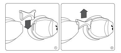
Snap the Smart Coach into the left lens of the Smart Goggle until you hear TWO "CLICKS". One "click" to position and one "click" to secure.
