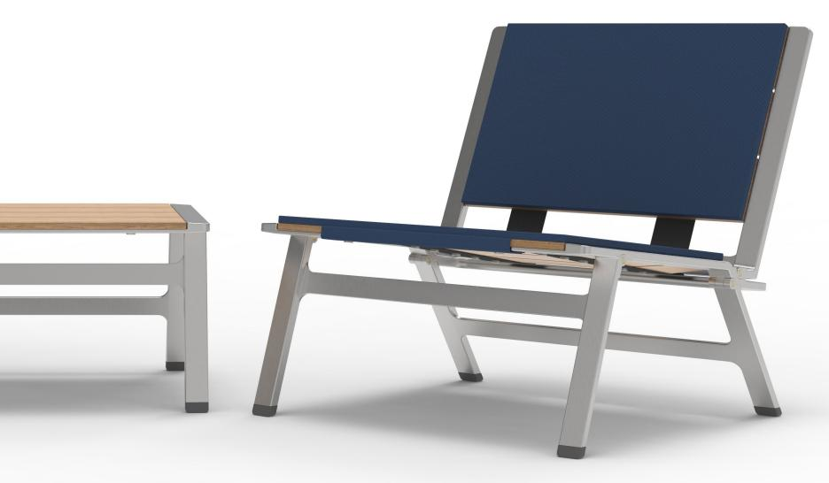
Teak wood slats are secured to webbing straps rather than the stainless steel frame to provide flex and added comfort in the seat. A jog in the seat frame creates a handle when folded and provides the needed geometry for an over center design that keeps the webbing in tension and the backrest open while in use.
