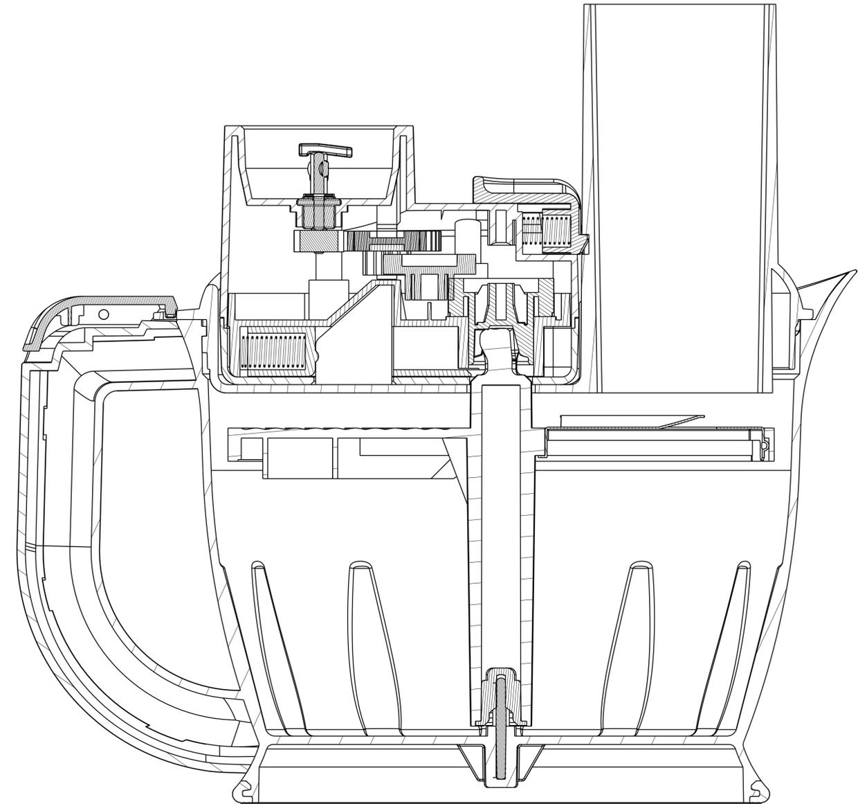
Thanks to patented gear box design on Lura hand blender , gearbox can be separated from lid easily with one click, and the lid can be washed through running water or even in dishwasher safely
