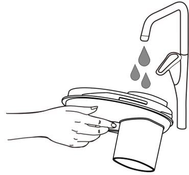
In traditional blender designs, the construction of the gearbox inside the chamber cover complicates the construction of the chamber cover and makes it impossible to clean the chamber cover easily under water.
