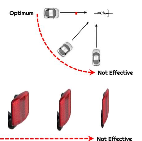
Reflectivity Is Minimised For Increases In The Observation Height Of The Approach Vehicle.
