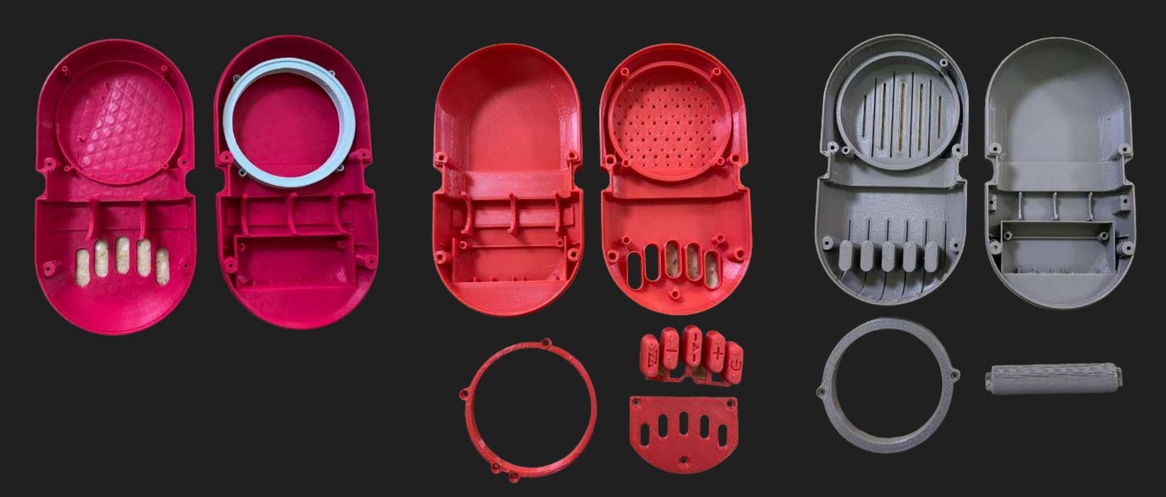
The developments started from left to right, from the **speaker** size and it's support, **battery** placement problems, and **chip** installation, and aesthetic buttons. Grey print is last **internal function development process**.
