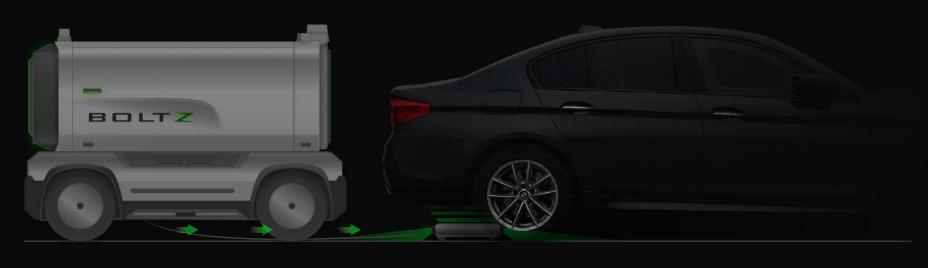
The robot aligns with the EV's wireless charging port and starts the wireless charging service.
