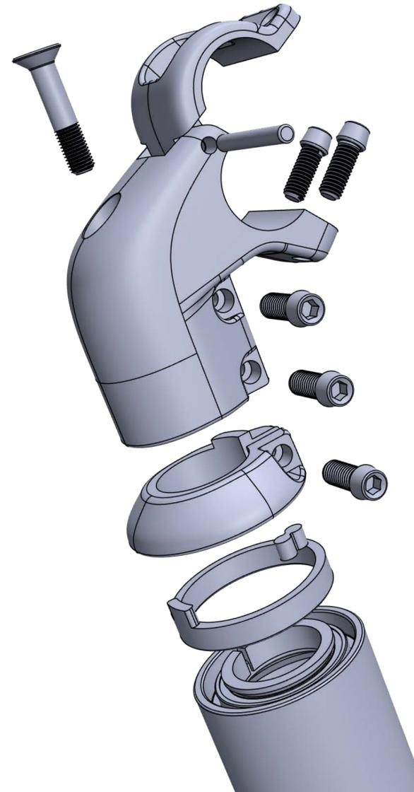
Our goal was to add a clamp for faster and easier assembly, move the bolts of the stem and clamp to the opposite side of the steerer tube for safety, and integrate internal cables and steering limiter inside the headset.
