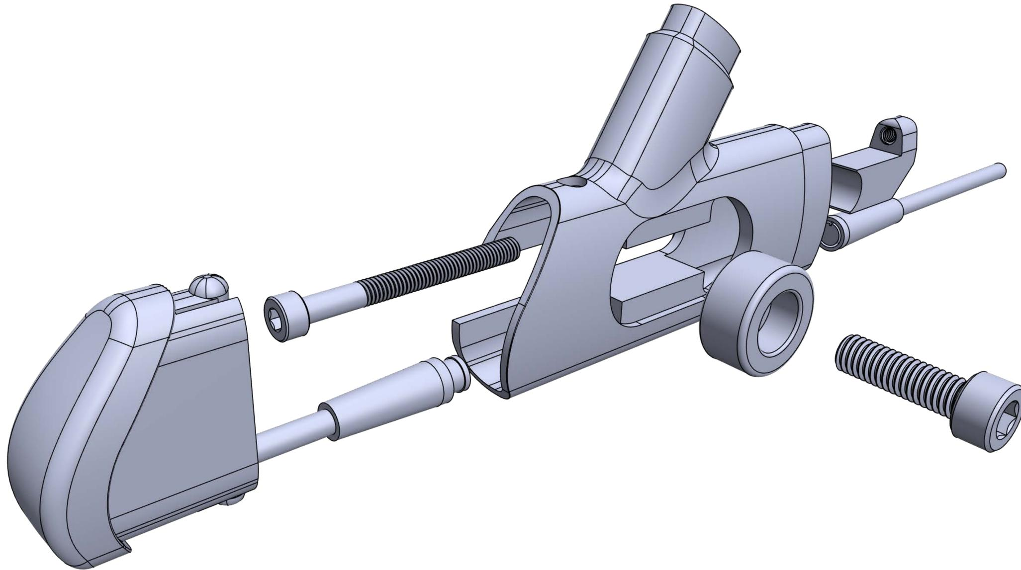
Our goal was to add into this dropout the lighting and internal cable, wheel mounting, and a chain tensioner.
