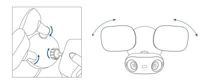
Note: \*Use the wrench to tighten or loosen the camera knob if needed.
