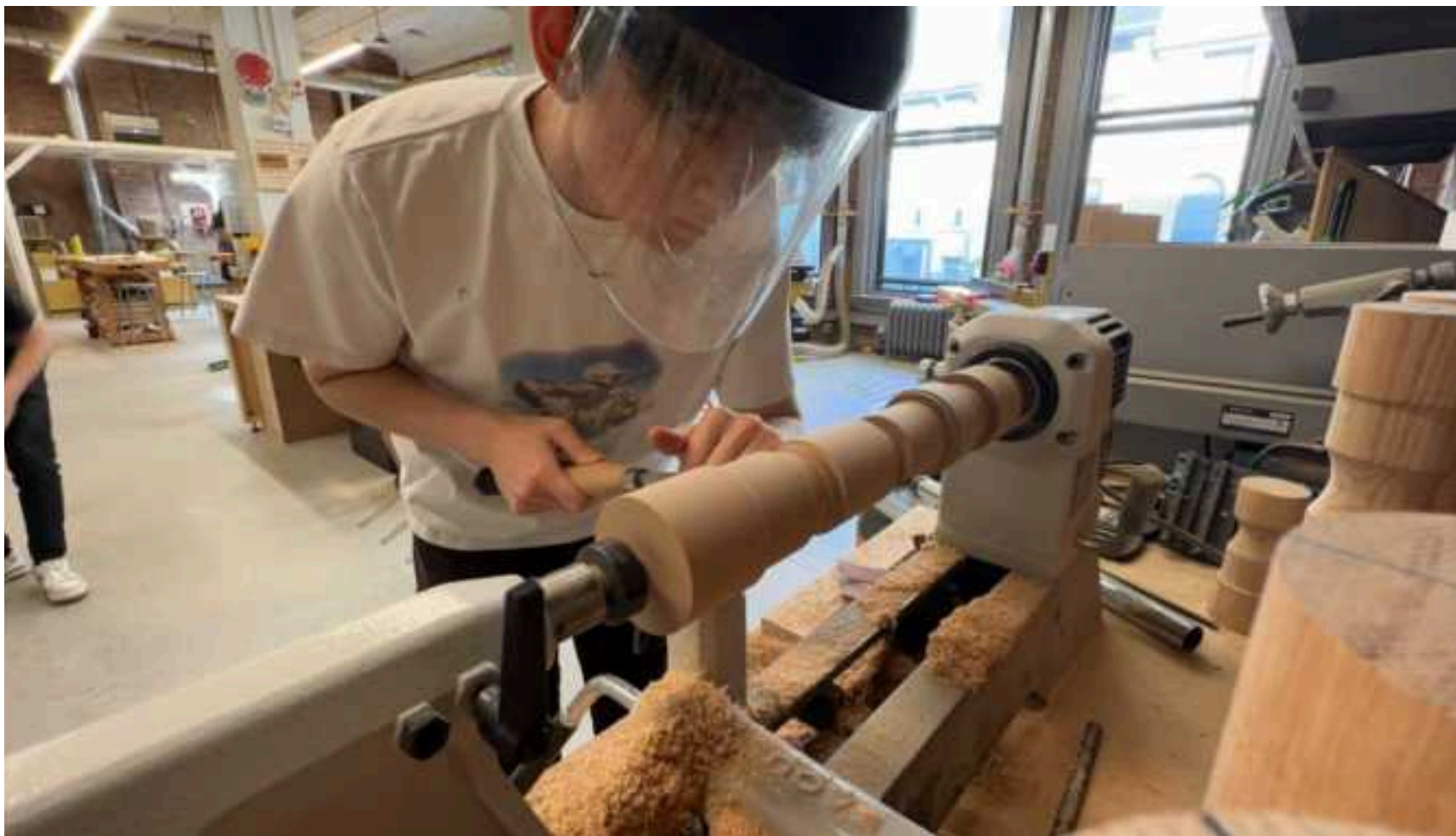
Rectangular cut out profile was carved to get the right dimension
