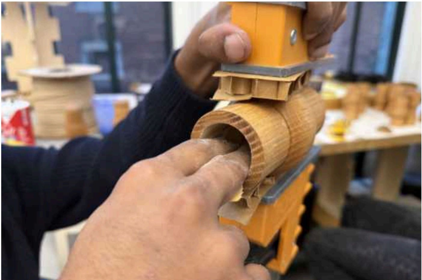
The routed cavity was sanded to obtain a smooth surface.
