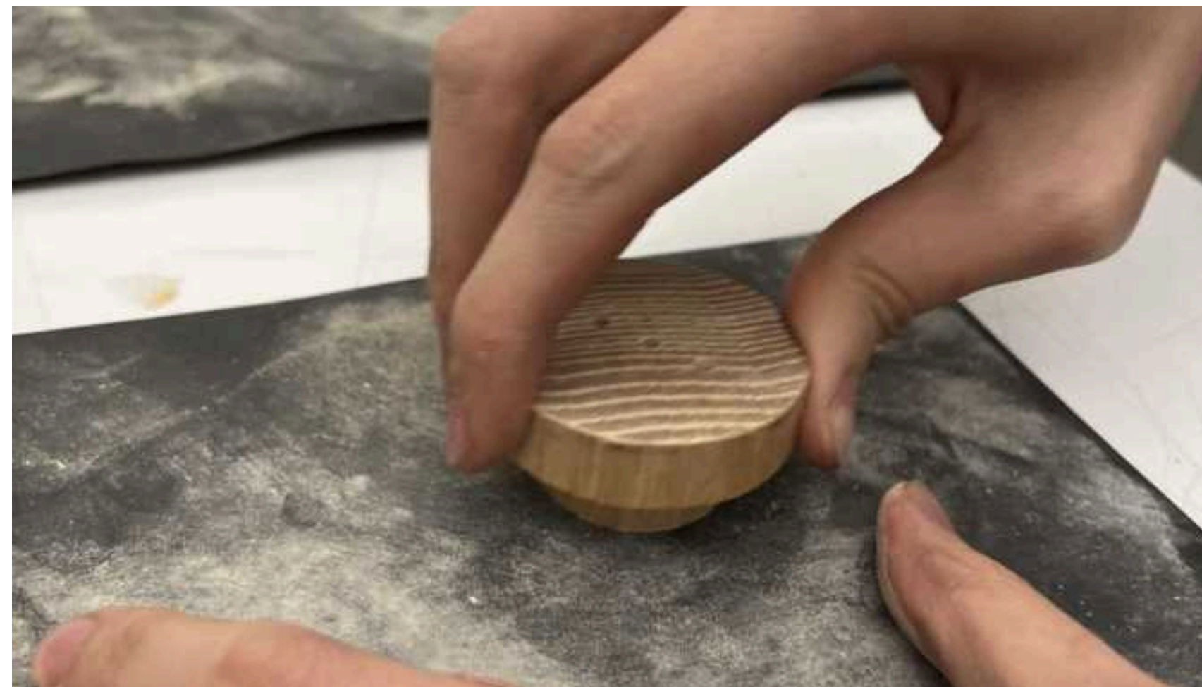
The caps were sanded to have a flat surface.
