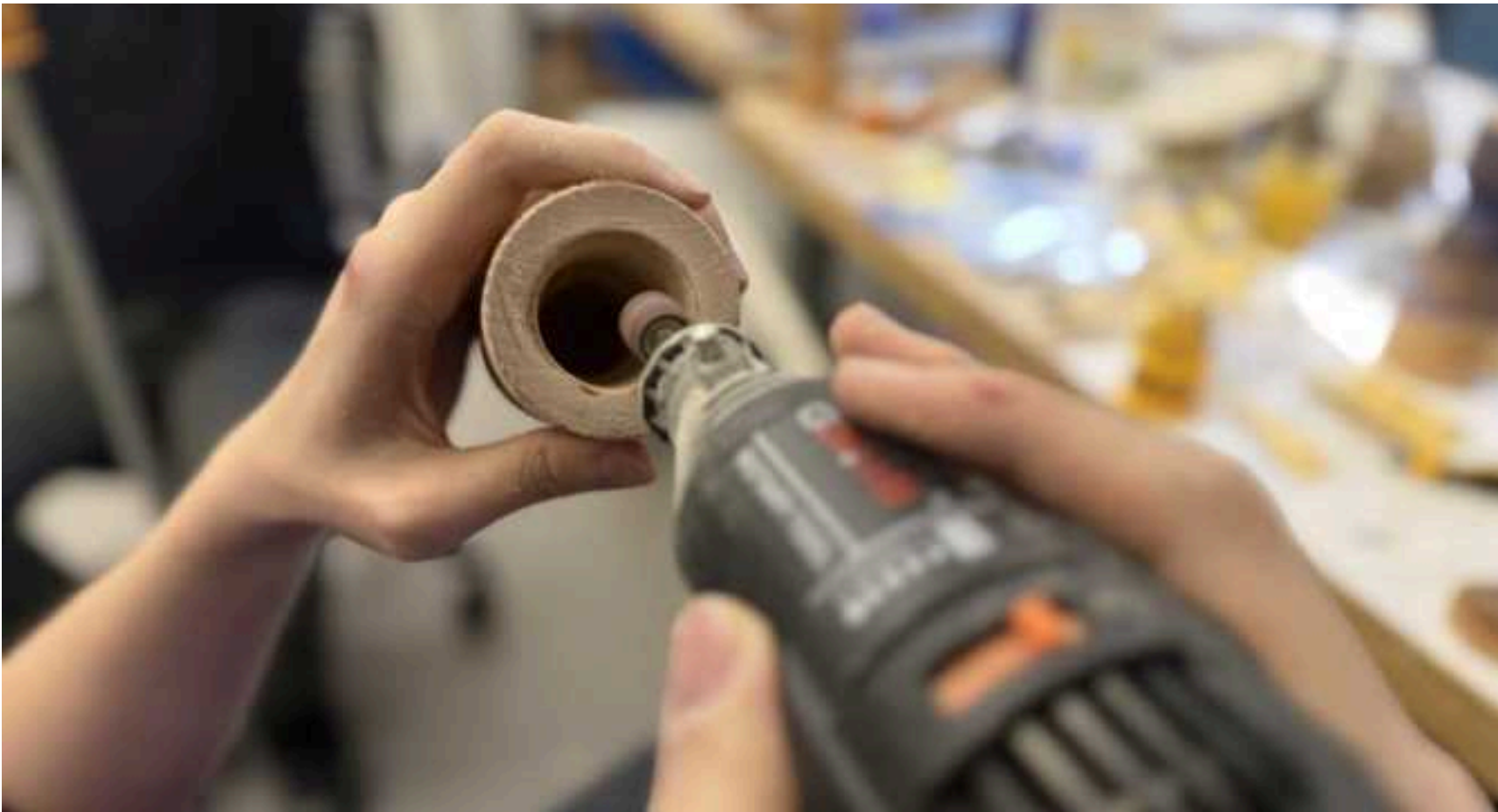
The shaker's cavity was routed for the lid to fit.
