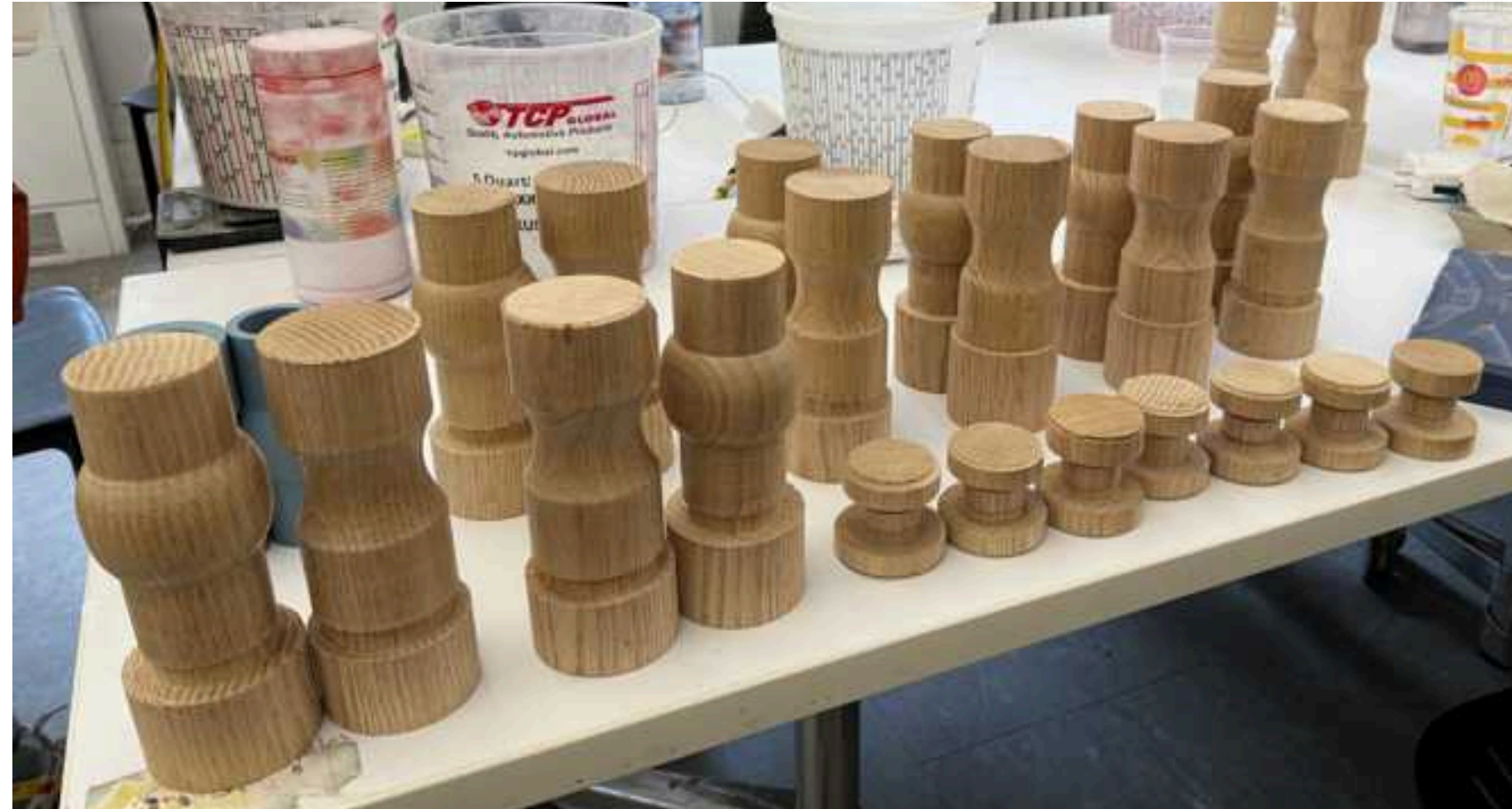
The polished blank was cut into individual shakers in the bandsaw.
