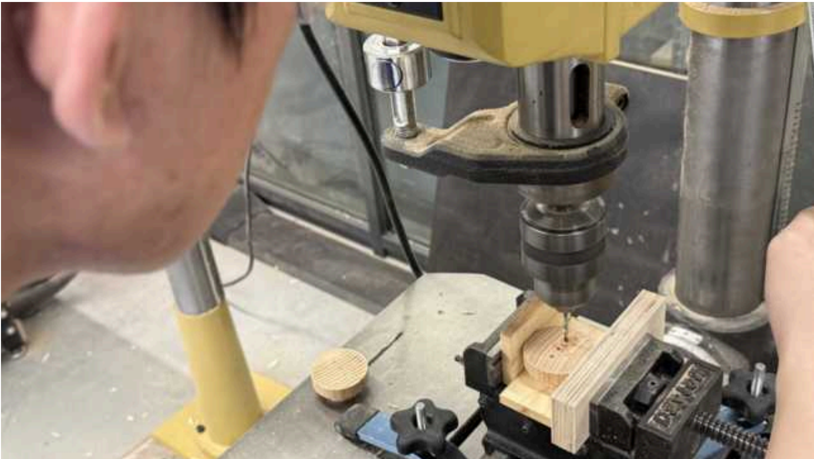
Pour holes in the lid were drilled using the drill press.
