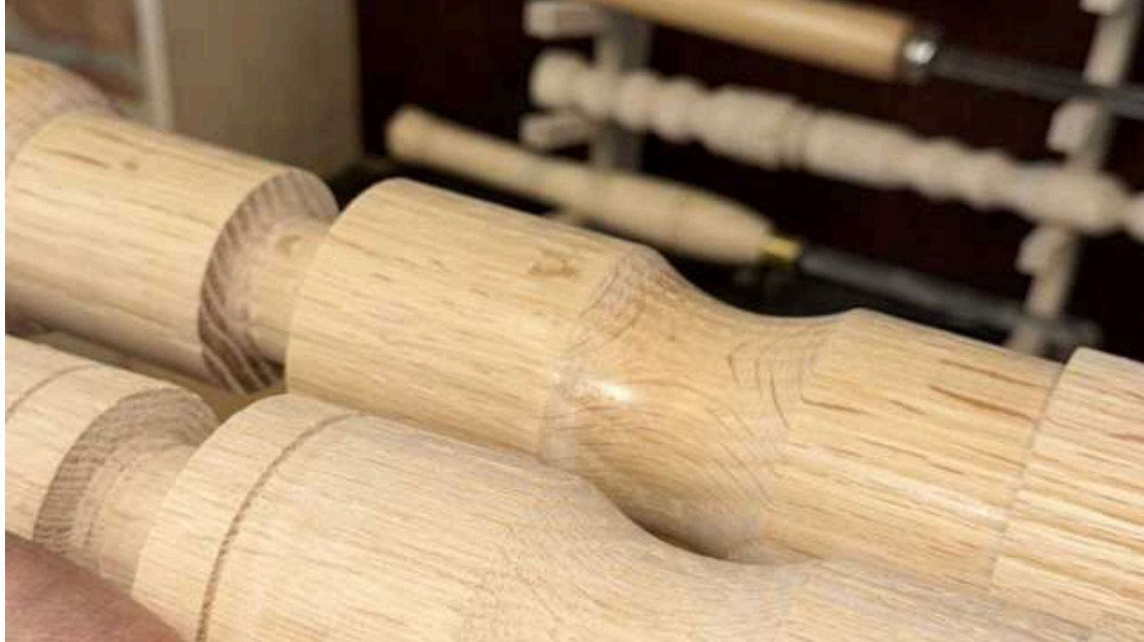
The turned blank was sanded to achieve a polished finish.
