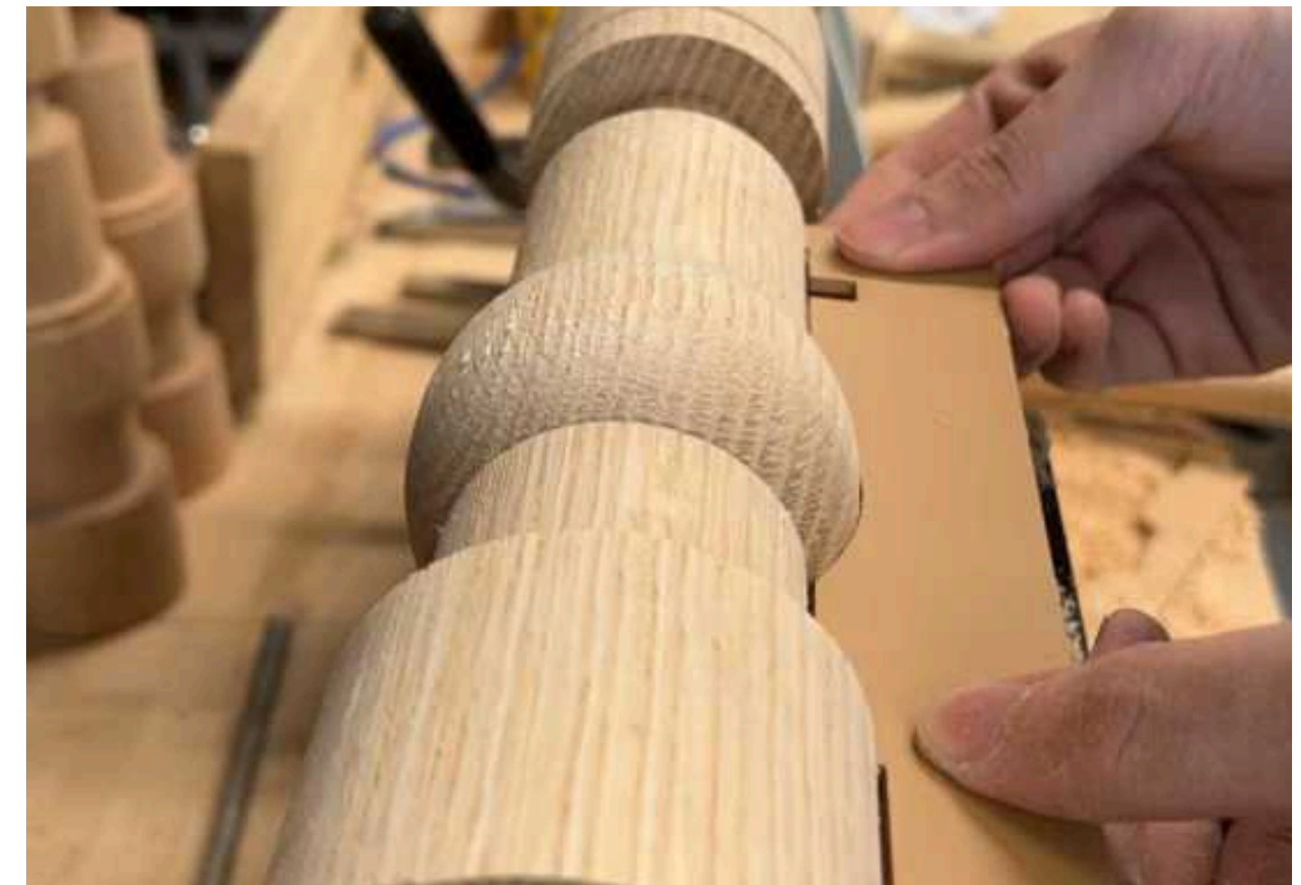
The sharp profile was then fillet turned to get the final shape
