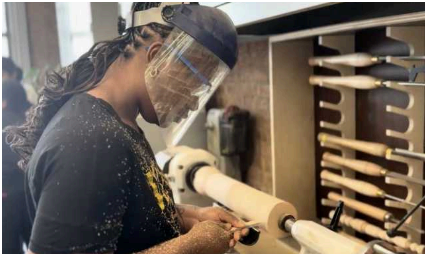
The roughing process created a cylindrical shape before adding details.
