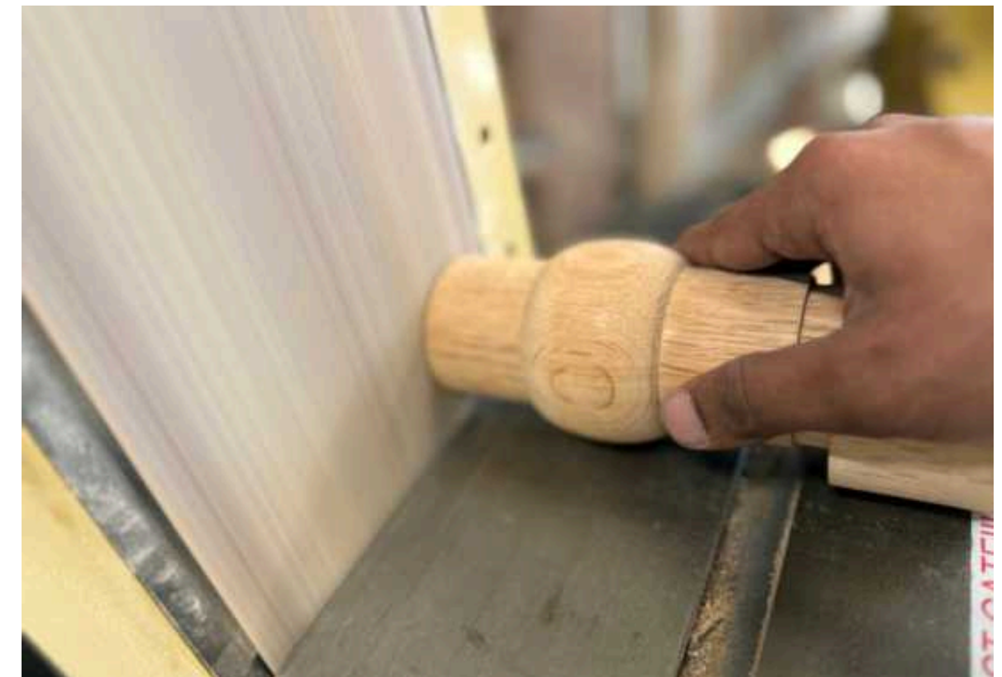
The shakers were simultaneously sanded for a smooth finish.
