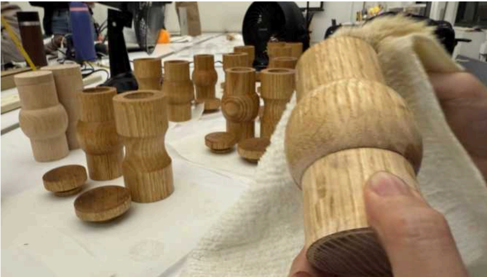
The final pieces were oiled with 2 coats of Tung Oil and set to dry.
