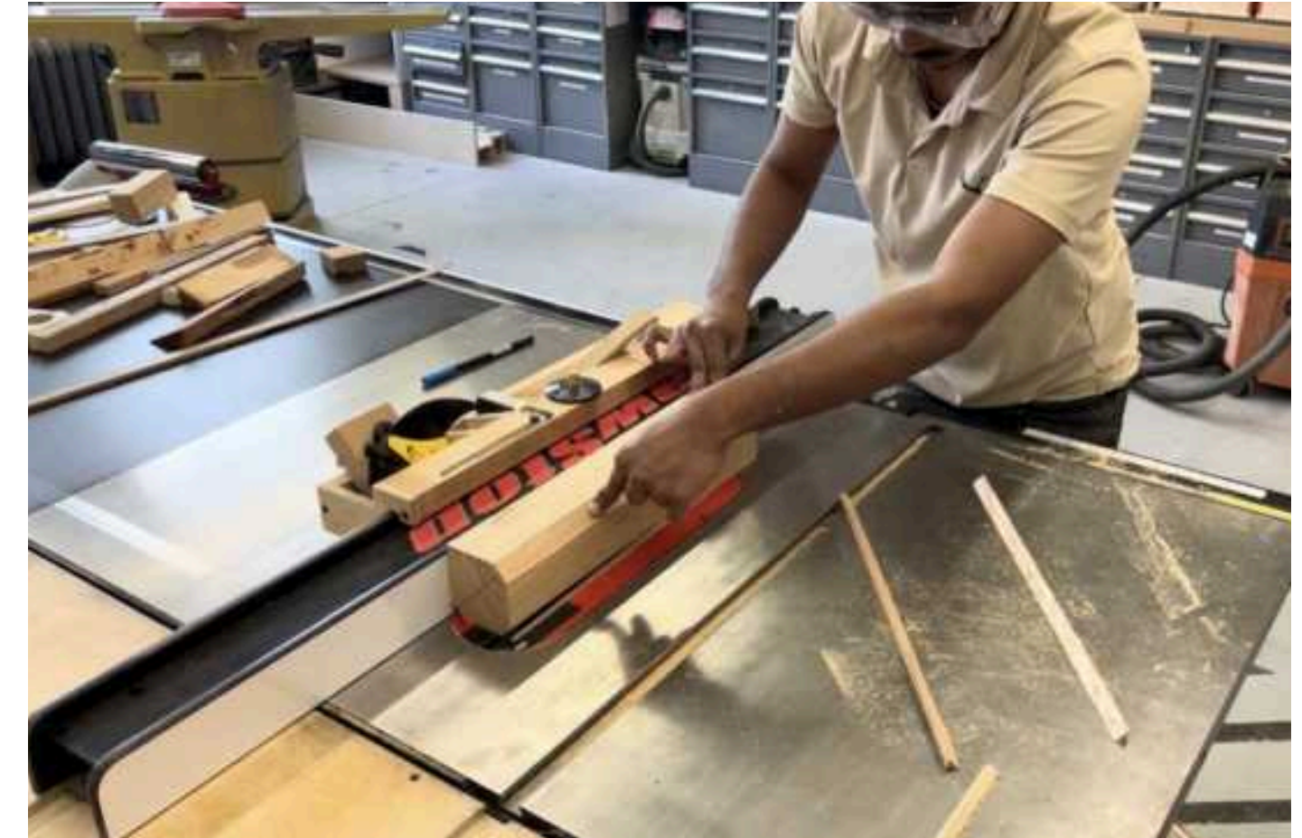
The blanks were chamfered to conduct roughing efficiently.
