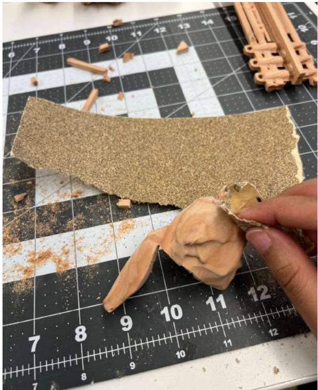
Smoothing surfaces with sandpaper (img. 53)
