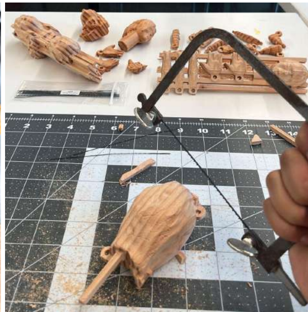
Jewelers saw for the finer cut (img. 52)
