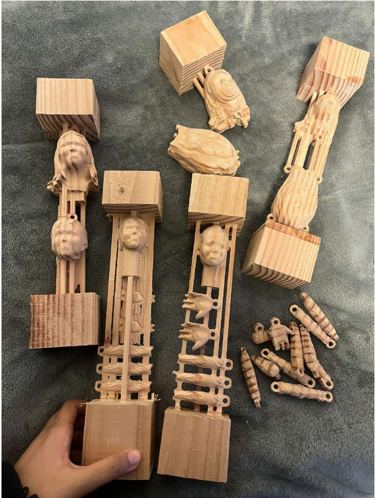
Final cuts from Roland CNC milling (img. 49)
