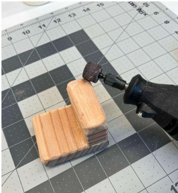
Sanding wood to curve the ends (img. 55)
