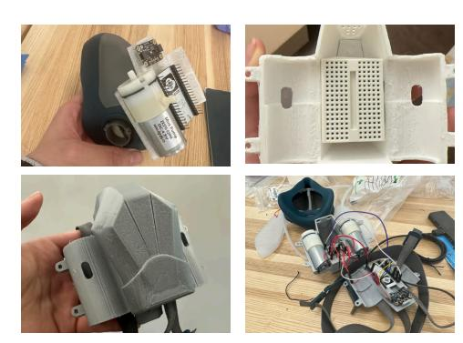
We molded silicone with 3D-printed molds to create the soft robotics part that attaches to the respirator. The shape resembles the theme of "lungs" and accurately blocks the airways when inflated.
