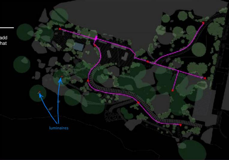
No problem, since poles act as premade installation manholes from which we can power additional luminaires
